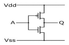
Figure 2.1 Basic CMOS cell
